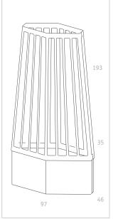
Mobile planter, galvanised sheet metal, powder-coated white, two fixed castors, two swivelling castors
